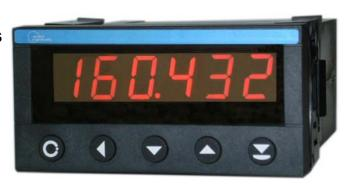
OC7040A-POL is a programmable 6 digit instrument with inputs for process signals such as 0-20mA, 4-20mA, 0-1V, 0-10V, -1V...+1V und -10V...+10VDC and 20mV Strain Gauge Applications. The display can be scaled in required process units like kg, gr, lb, kN etc. Isolated excitation is available for supplying of external sensors. Output options Set Points, Analog Outputs and Serial Data Ports are suitable for control applications.
